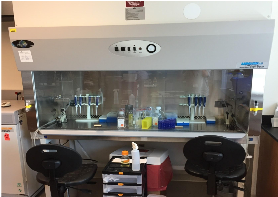
Figure 7.4: A biosafety cabinet at the Burnett School of Biomedical Sciences. Notice the ethanol spray bottle and the pipettes used for preparing the samples.
