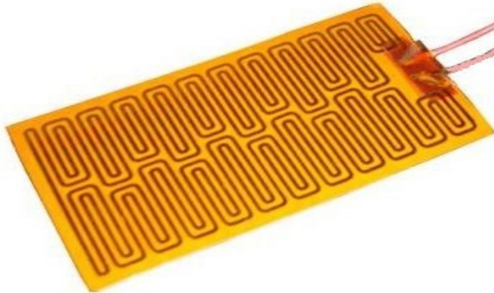
Figure 5.3: Kapton heating element
