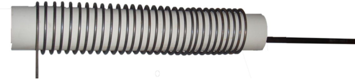
Figure 5.2: Kanthal heating element example
