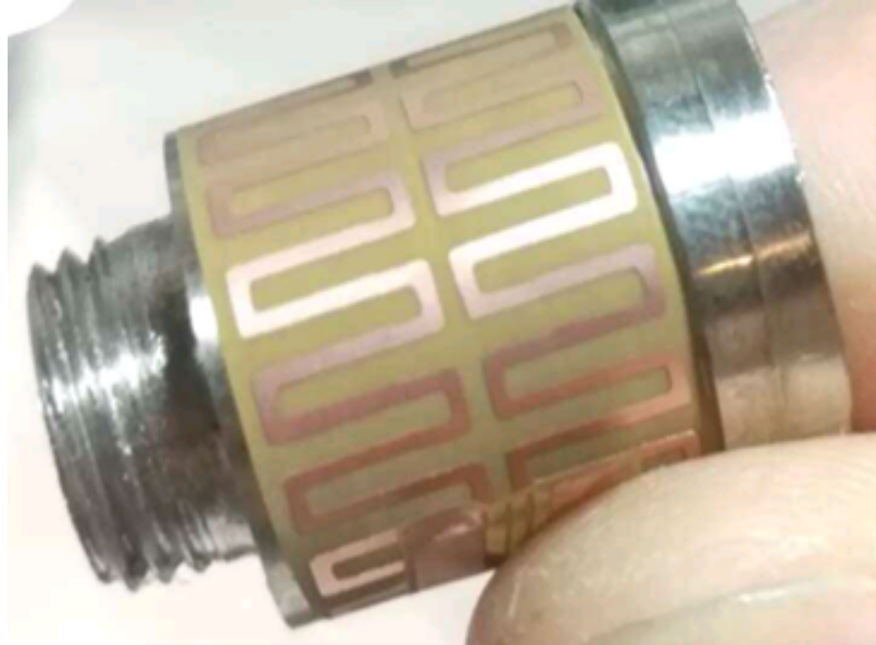
Figure 6.4: Etched Kapton Heating Element
